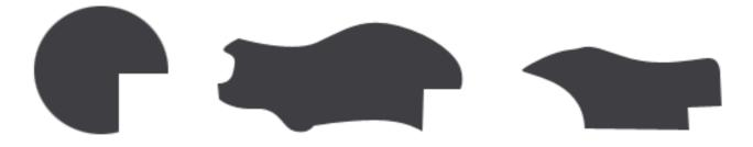
Examples of round or exaggeratedly misshapen mouldings or mouldings with no proper heel, which must not be cut by the CS 939 and the CS 939MA.
